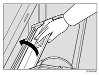
**3** If you could not remove the misfed master in steps **1** and **2**, pull out the drum and remove the misfed master from the inside.
